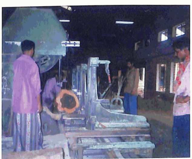
Plate 4. Conversion of log to small clear specimens
