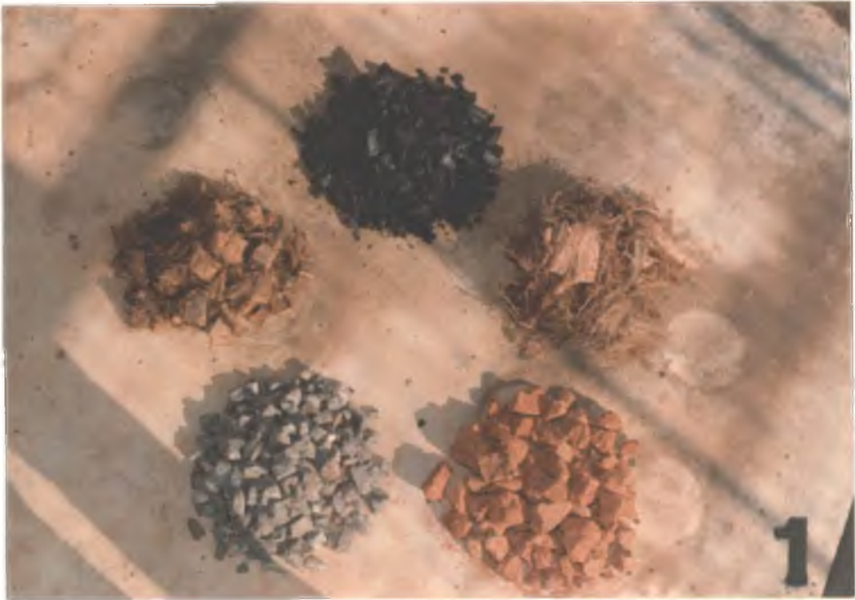
Clock wise from top - Charcoal, coconut fibre, brick, gravel and husk
