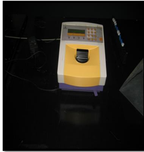
Plate 6. Liquid scintillation counter Hidex Triathler Multilabel tester used for recording the radioactivity in tissues
