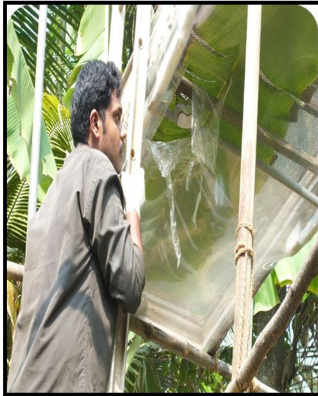
Plate 7. Suspending the crucible inside the leaf chamber below the mid part of the adaxial side of the leaf using a wire mesh
