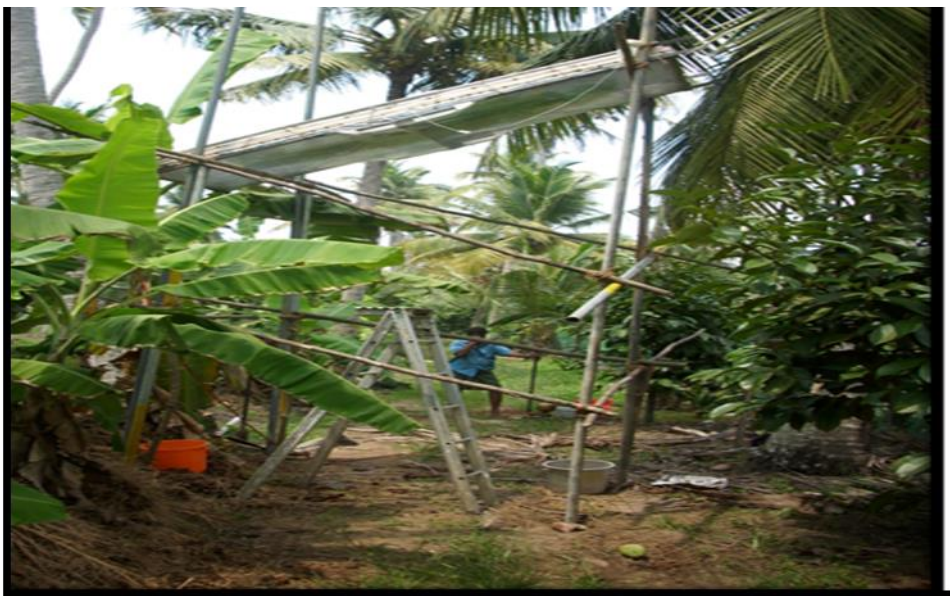
Plate 2. Leaf chamber placed in correct orientation of leaf for feeding of CO 2
