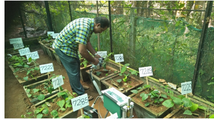
Measurement of Physiological parameters with IRGA
