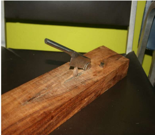
Plate 1. Nutcracker designed for seed extraction
