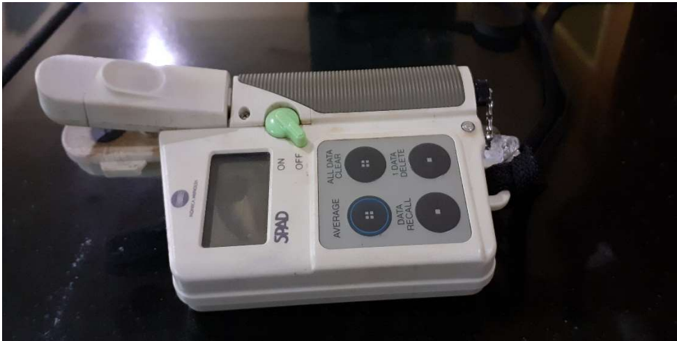
Plate 5. SPAD meter to measure the chlorophyll content of the leave
