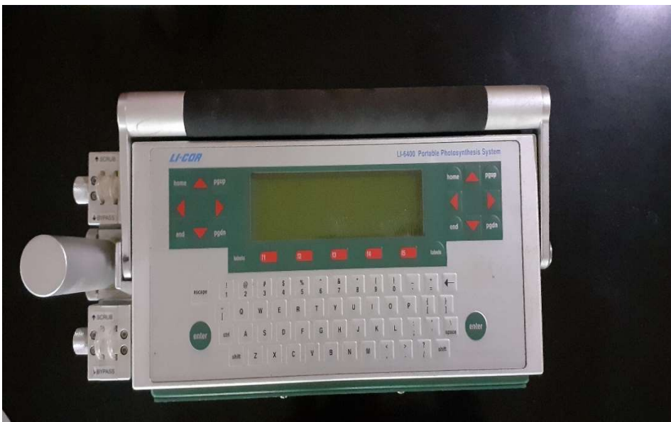
Plate 6. Infrared gas analyser used for measuring physiological attributes
