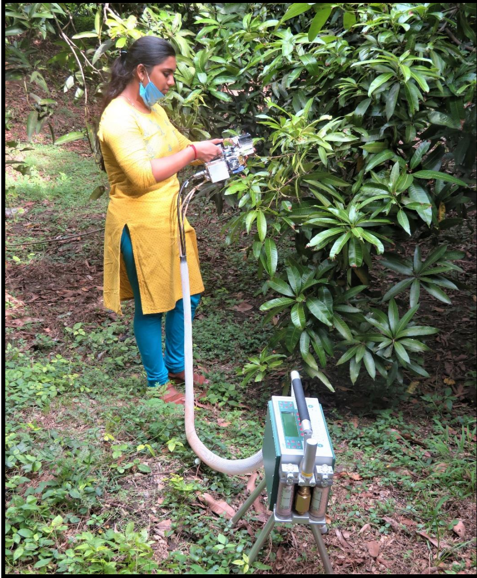
Plate 18. Observations on stomatal conductance, photosynthetic and transpiration rate using IRGA
