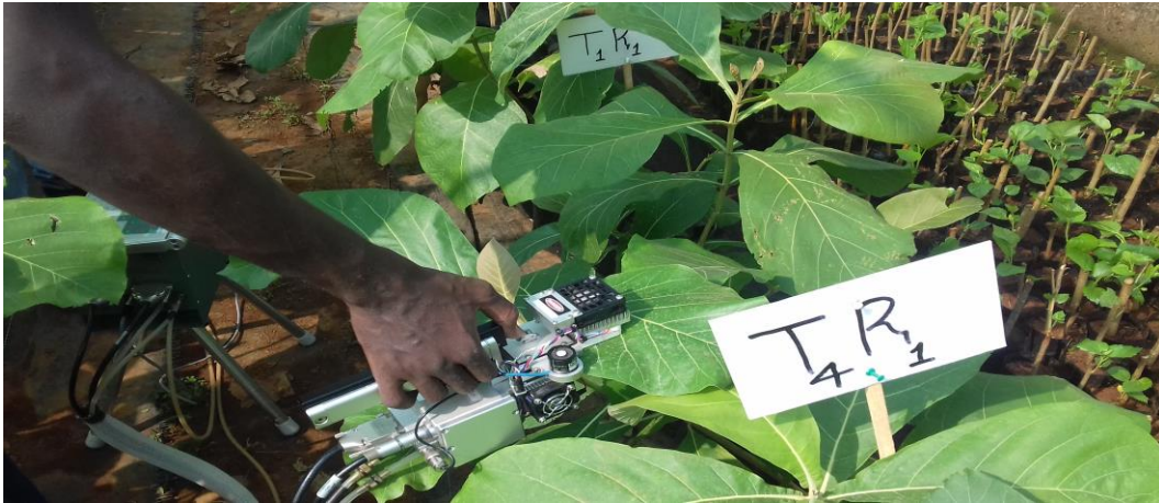
b. Measuring gas exchange parameters using IRGA
