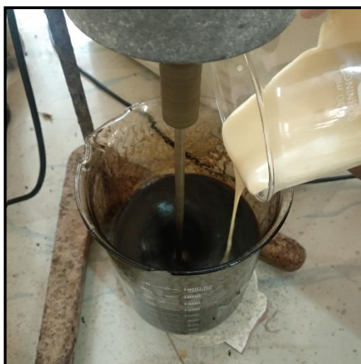
C. Blending mixture of emulsifier with solvent and cosolvent
