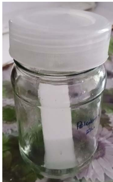
Plate 4. Glass slides dipped in a bottle containing petroleum ether
