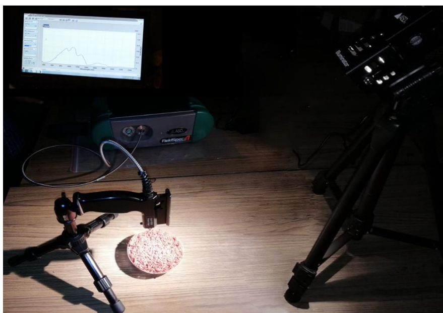
Plate C1. Spectra acquisition using ASD FieldSpec-4 spectroradiometer
