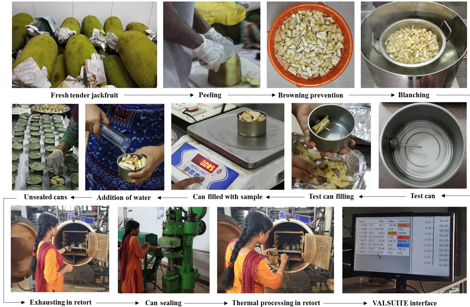
Fig. 3.1 Steps involved in thermal processing and canning of tender jackfruit
