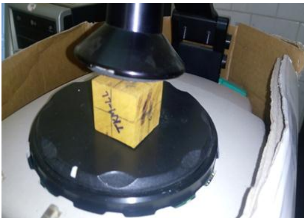
Plate 5: Color determination of Artocarpus heterophyllus wood samples by using Hunter Lab Scan XE colorimeter (IWST, Bangalore, Karnataka)
