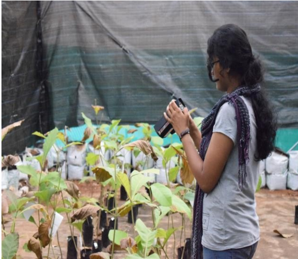
Measuring CATD using Infrared Thermometer
