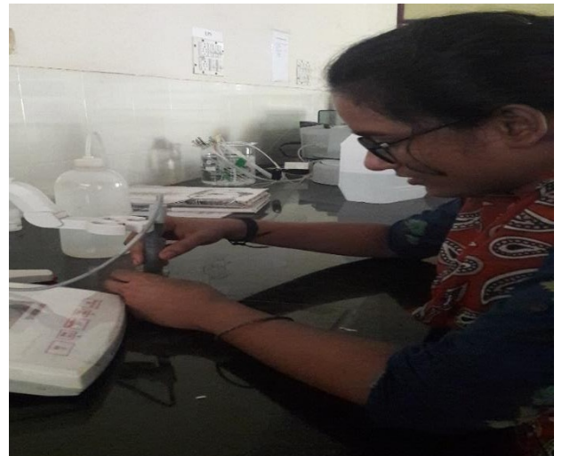
Measuring membrane stability index using conductivity meter
