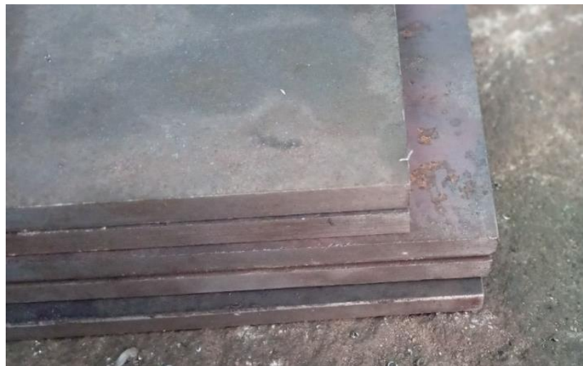
Plate 3.14 Mild steel plate of 12mm thickness
