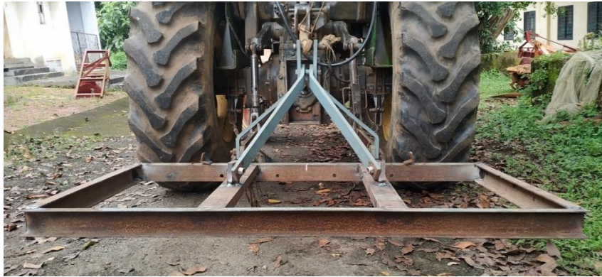
Plate 3.5 Lowest reach position of tractor lower links
