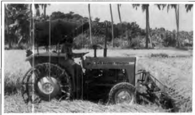
Plate 49. Tractor mounted paddy reaper windrower
