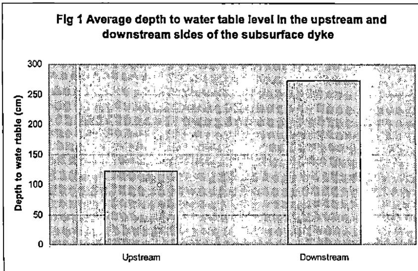
consequence of the obstruction of the runoff seepage losses of soil moisture. The plastic sheets in the dyke obstruct the flow of sub-surface water raising water table in the catchment area. The existing pond in the upstream side of the dyke which usually gets dried up in summer is now maintaining higher water table throughout the year as the dyke ensures incessant supply of water to the pond.
