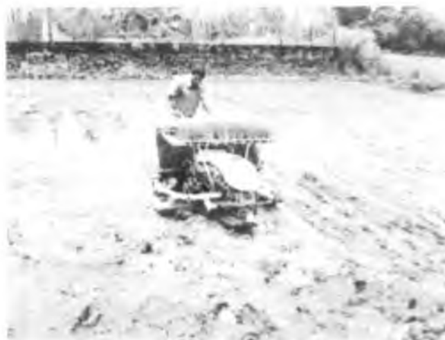
Figure.3 Trial tests of walking type rice transplanter at RRS, Vytilla for pokkali
