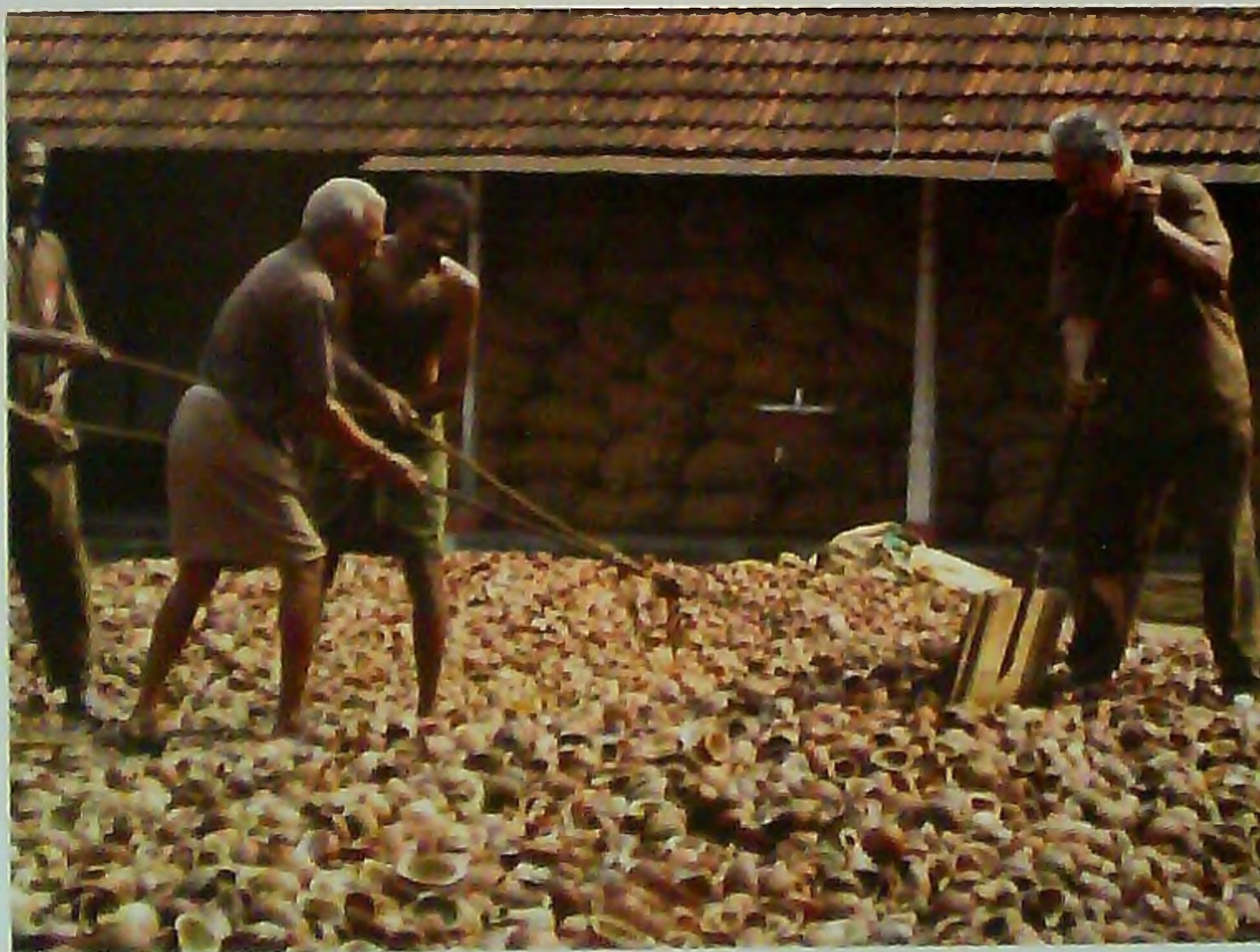
Figure 10. Copra making by solar drying
