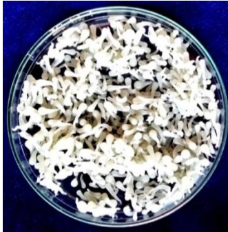
Beads prepared from 3.5 % sodium alginate solution with additives
