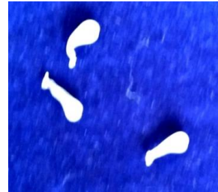
Beads prepared from 3.5 % sodium alginate solution with additives
