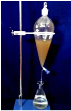
Bioagent amended sodium alginate solution taken in a separating funnel
