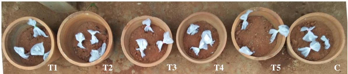
Beads in nylon bags buried for degradation study
