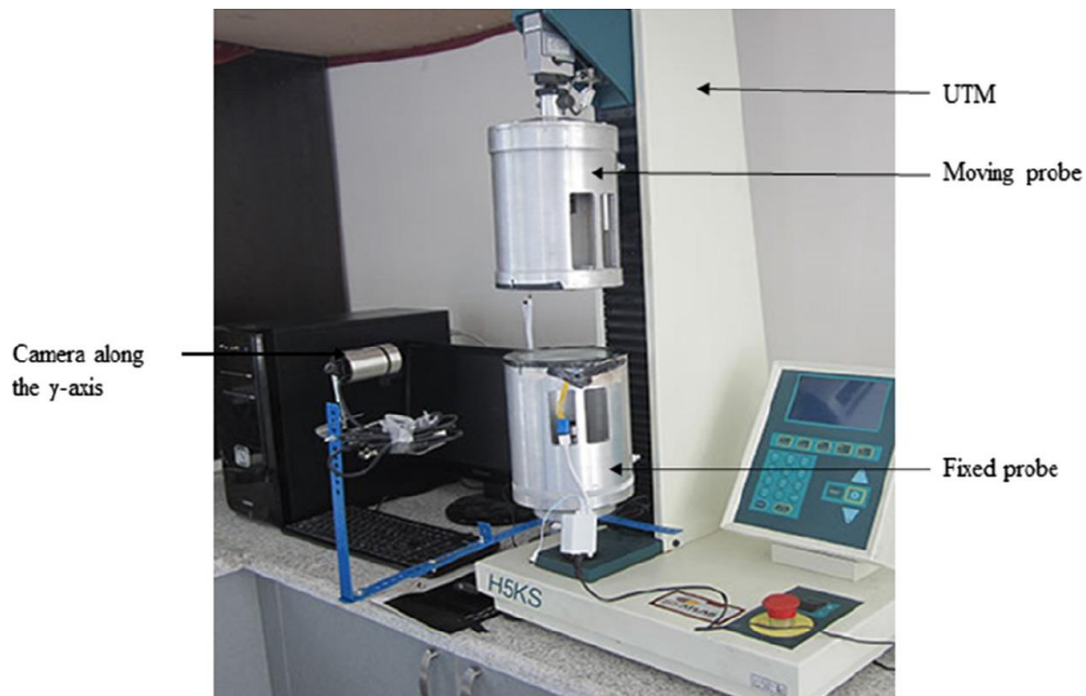
Figure 2.3 Probe and camera setup (Malekabadi et al. , 2017)
