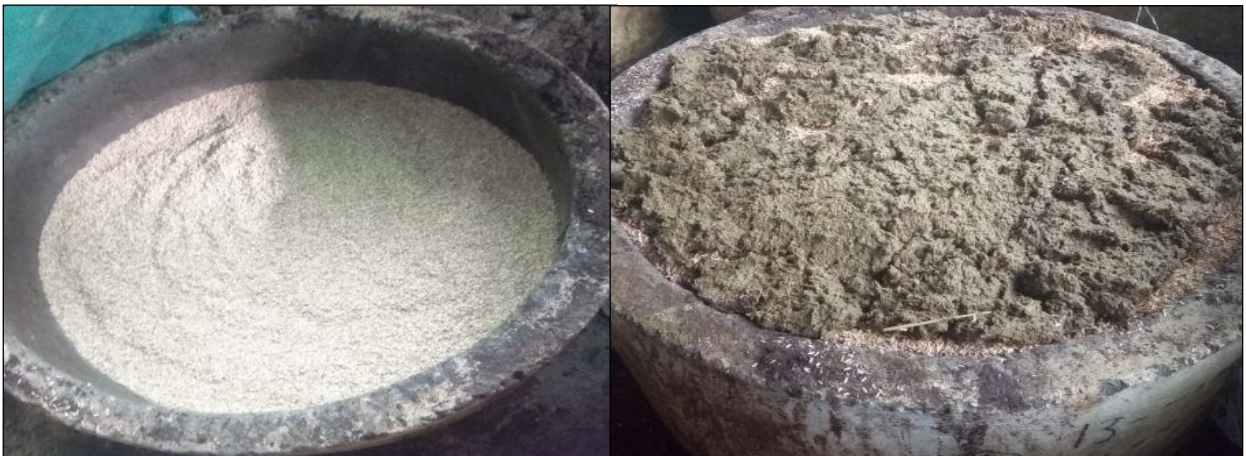
Plate 3.5: Filling rice husk and cowdung in alternate layer
