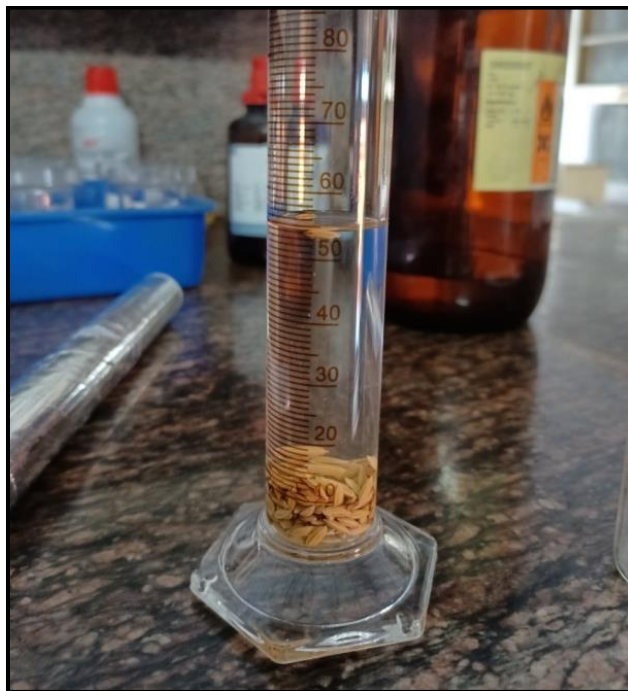
Plate 3.5 Volume determination of pokkali paddy (‘ Vytilla - 1 ’ variety) using Toluene displacement method
