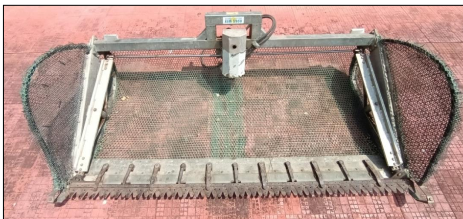
Plate 3.3 Amphibian Weed Harvesting Attachment
