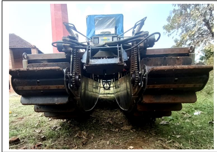
Plate 3.2 Rear view of Truxor DM 5045 showing Track belt – Grousers – Pulley drive
