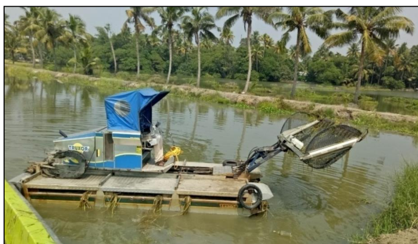
Plate 3.4 Amphibian Weed Harvester (Truxor DM 5045)
