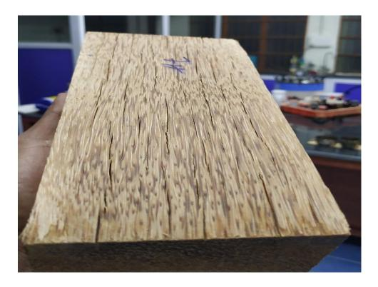
Plate 3.2. Surface check observed during initial stage of quick drying test of 50 mm thick high-density coconut palm wood
