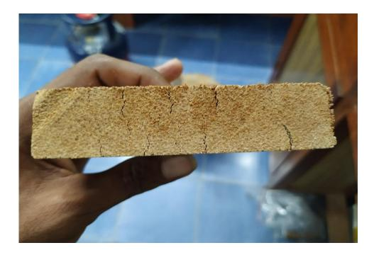
Plate 3.1. End check observed during initial stage of quick drying test of 25 mm thick medium-density coconut palm wood
