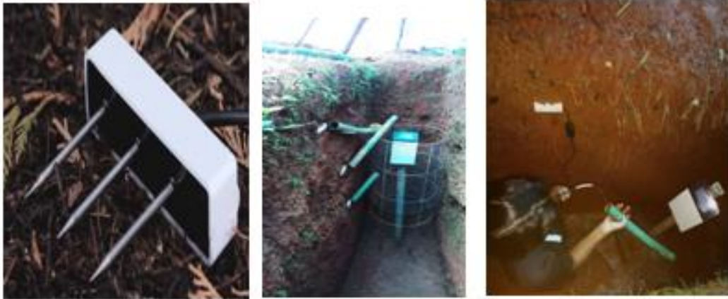
Plate 3.2 Installation of TEROS12 sensors in field for reliability check before calibration
