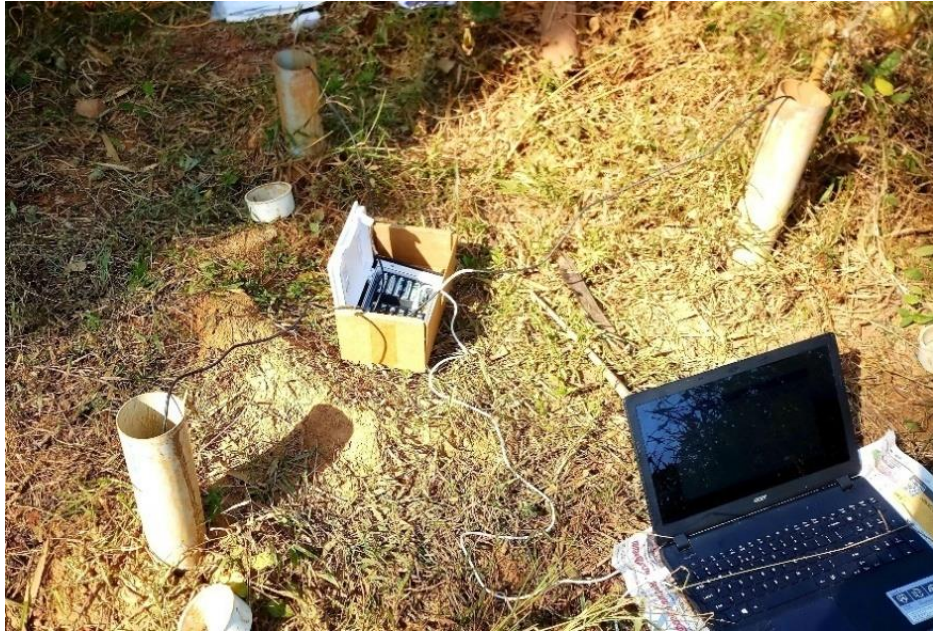
Plate 3.5 Monitoring of base flow through salt tracer analysis and TEROS12 measurements
