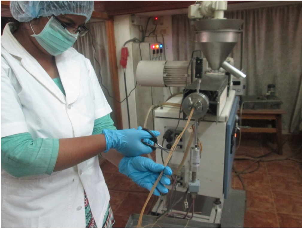
Extrusion of noodles
