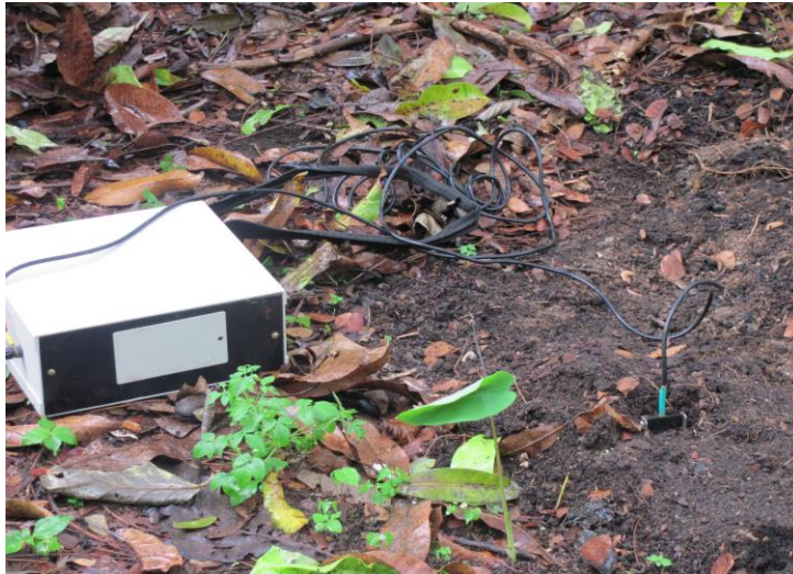
Plate 3. Moisture measurement with moisture metre
