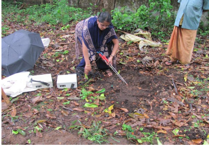
Plate 2. Temperature measurement with multi channel temperature recorder
