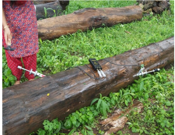
Plate 24. Measurements taken in teak ( Tectona grandis ) log having hollow inside by inserting the transducers at 1 m interval on the opposite side of the log
