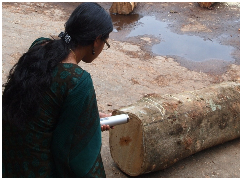
Plate 6. Measurements taken in rubber ( Hevea brasiliensis ) using pilodyn
