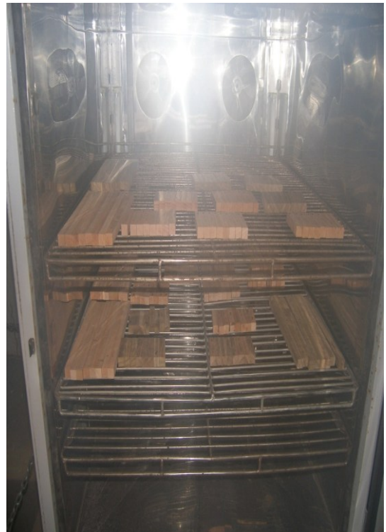
Plate 15. Wood samples kept for conditioning
