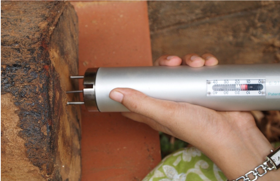
Plate 3. Using pilodyn for indirect assessment of density in species
