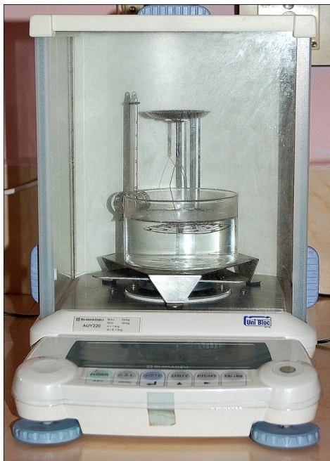
Plate 12. Specific gravity module attached to electronic balance (Shimadzu AUY 220)
