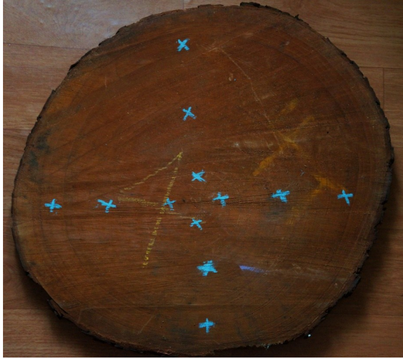
Plate 5. The positions at which measurements were taken at the end cross section of log using pilodyn
