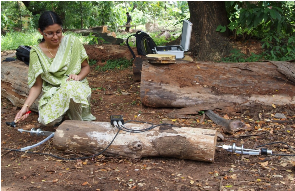
Plate 8. Measurements taken in teak ( Tectona grandis ) log using treesonic microsecond timer
