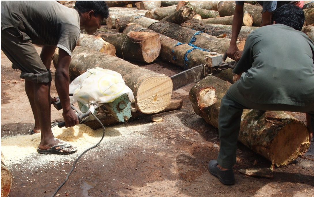
Plate 2. Crosscutting of discs of species to desired size
