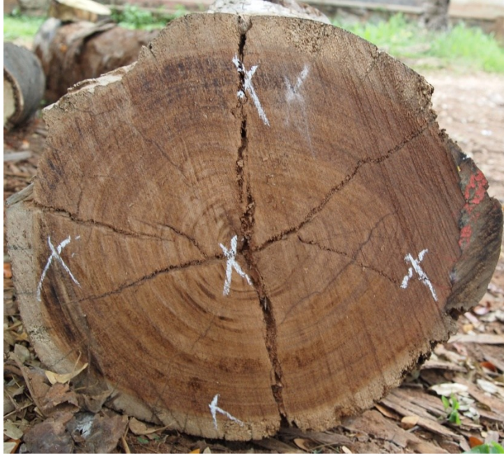
Plate 9. Positions on the end cross section of log at which measurements were taken using treesonic microsecond timer
