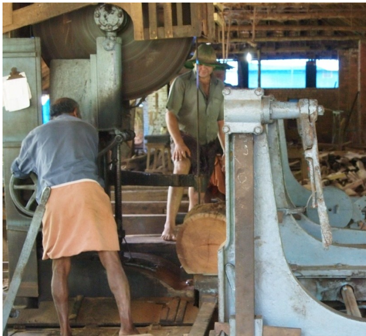
Plate 10. Conversion of logs to planks before making them to small clear specimens
