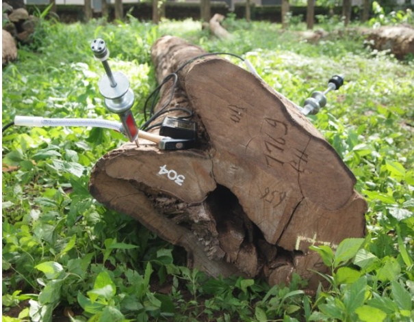
Plate 24. Measurements taken in teak ( Tectona grandis ) log having hollow inside by inserting the transducers at 1 m interval on the opposite side of the log
