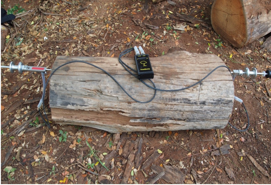
Plate 7. Start and stop transducers inserted into a pyinkado ( Xylia dolabriformis ) log
