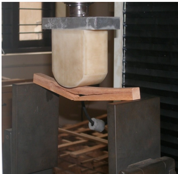
Plate 16. Static bending test parallel
