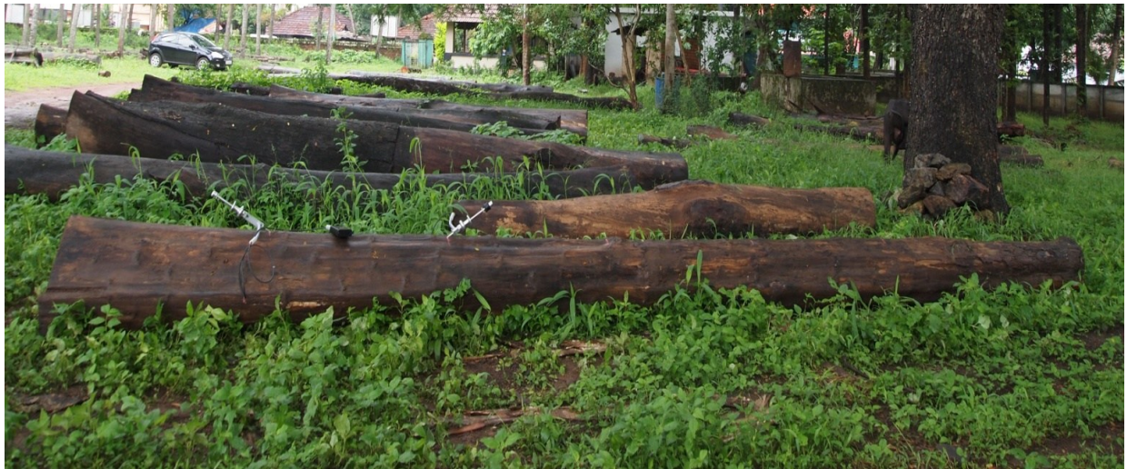
Plate 23. Measurements taken in teak ( Tectona grandis ) log having hollow inside by inserting the transducers at 1 m interval along the same side of the log
