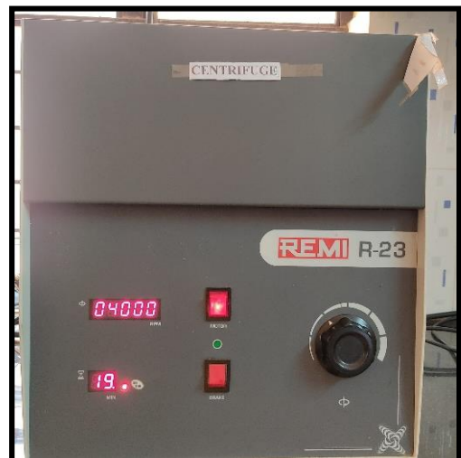
d. Centrifugation at 4000 rpm, 20 min
