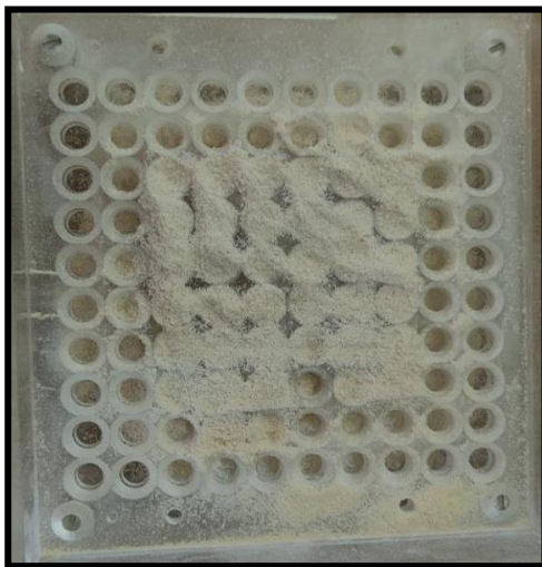
c. Placement of filler material
