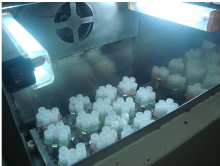
PLATE 4. Samples in orbital incubator shaker for adsorption study
