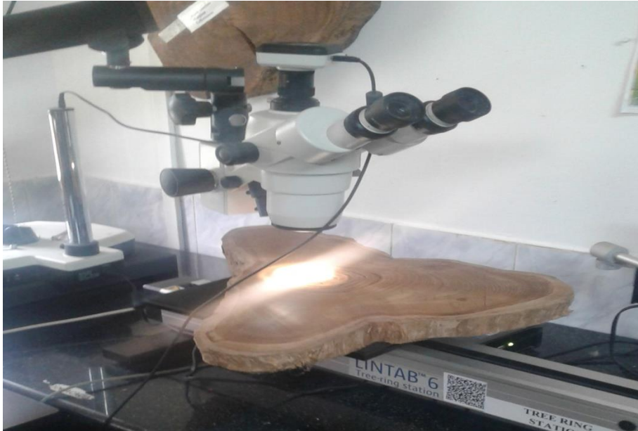
Figure3: Measurement of sample ring width using LINTAB – 6 at COF, KAU at Thrissur.
