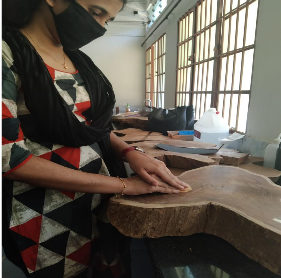
Figure2: Sample Preparation by smoothening process using sand paper
