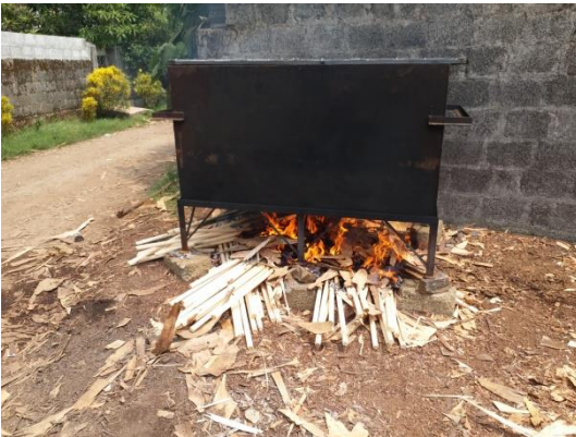
Plate 3: Pretreatment of coconut log
