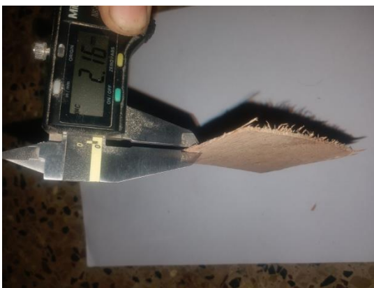
Plate 11: Thickness measurement of veneer using Digital Vernier calliper
