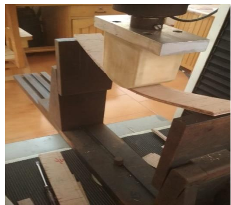
Plate 12: Static bending test of coconut plywood
