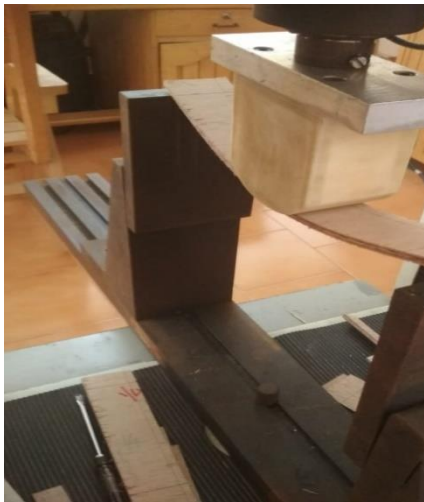
Plate 22: Static bending test of coconut plywood
