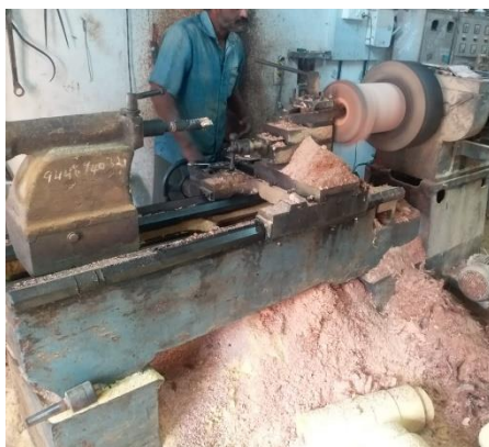
Plate 13: Lathe for boring coconut log
