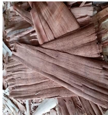
Plate 18: Example of collapsed veneer
