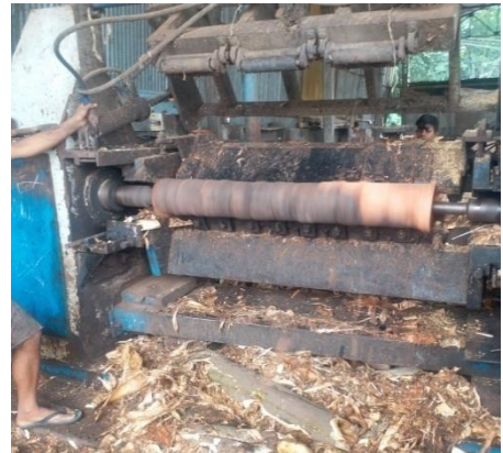
Plate 4: Debarking of coconut log
