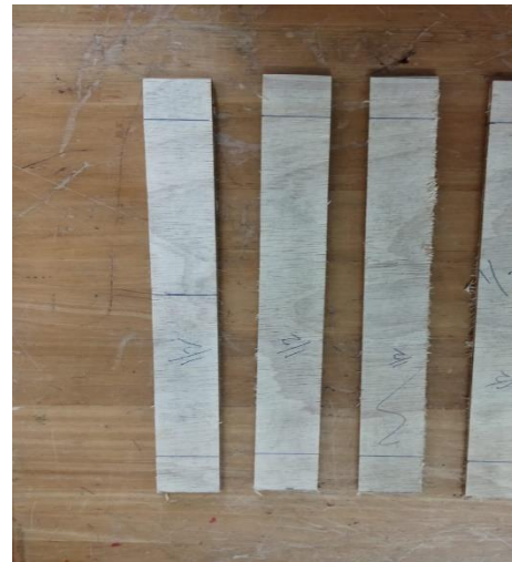
Plate 23: Samples of testing bending test parallel to face veneer of coconut plywood.
