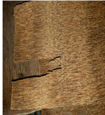
Plate 21: Example of veneer tear-out
