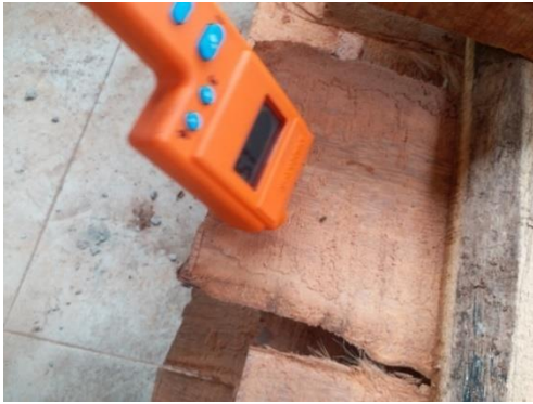
Plate 7: Moisture content analysis using moisture meter
