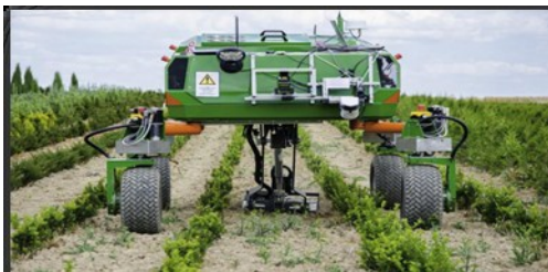
Plate 2. Weed controller Robot
