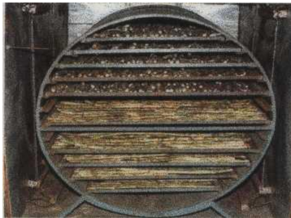
PLATE 1: Aerated steam treatment chamber
