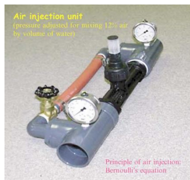
Figure 2. Air injection unit
