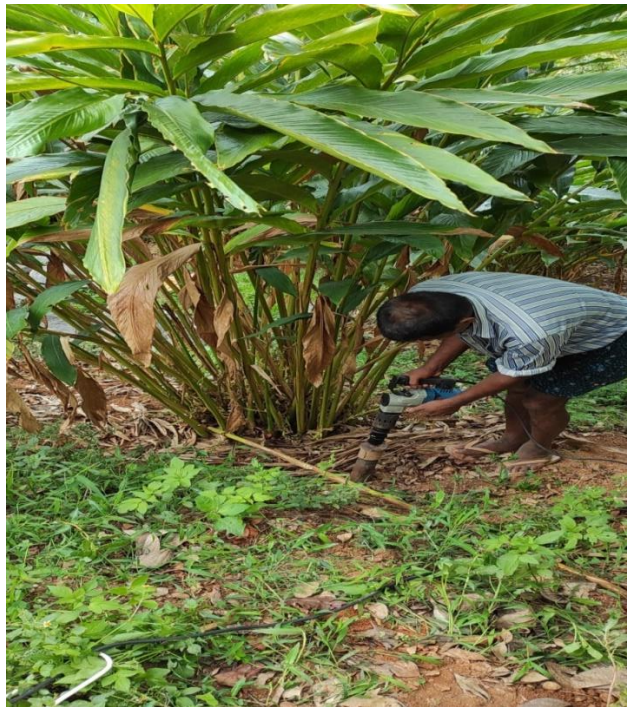
Plate 3. Soil sampling using soil sampler
