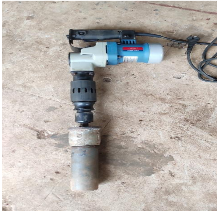
Plate 2 . Soil sampling machine when all parts are assembled
