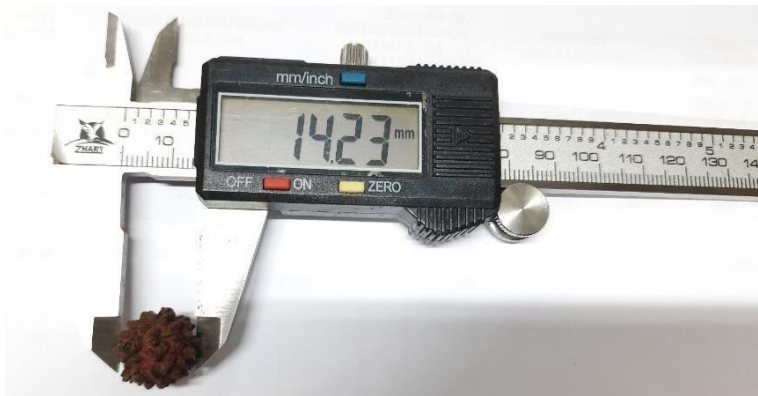
Plate 4. Measuring diameter of longan fruit using digital vernier caliper
