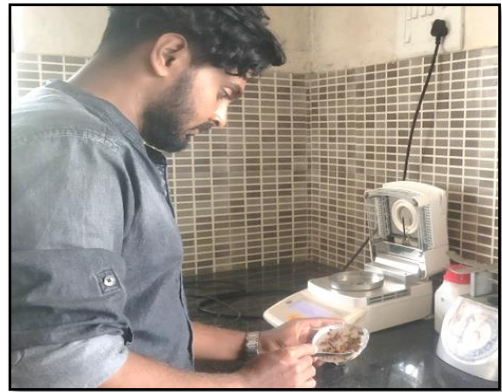
4b. Placing of sample in moisture analyser
