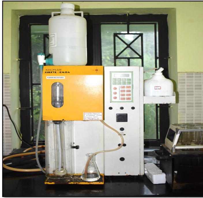
Plate 9. Analysing protein content of hive stored pollen sample
