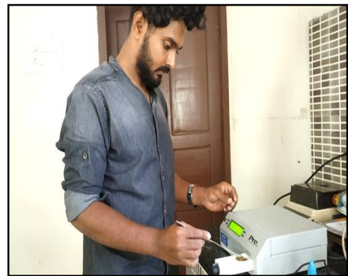
5b. Placing of sample in Water activity analyser
