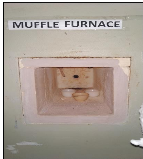
7b. Placing of samples inside Muffle furnace
