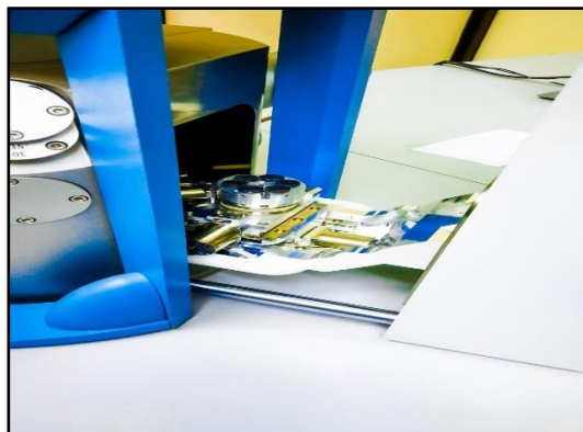
3c. Placing of Sputter coated pollen samples in SEM
