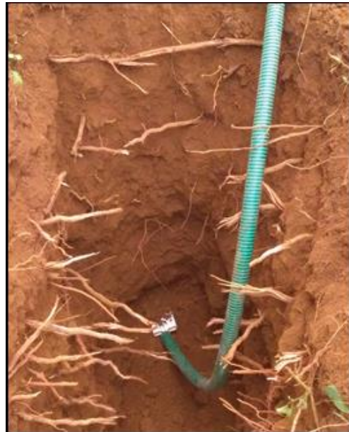
Fig. 3.19. CS650 Installed in the Study Area
