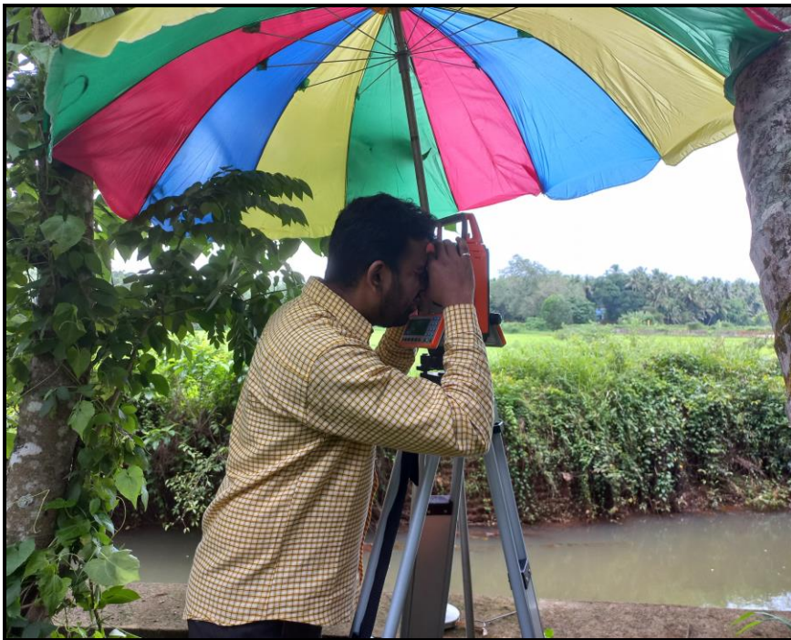
Fig. 3.9. Determination of Channel Cross-section using Total Station
