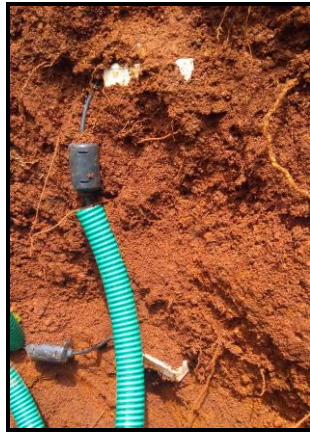
Fig. 3.14. TEROS 12 Soil Moisture Sensors Installed in the Study Area
