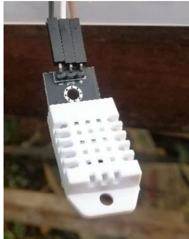
Plate 3.2 DHT22 temperature & humidity sensor
