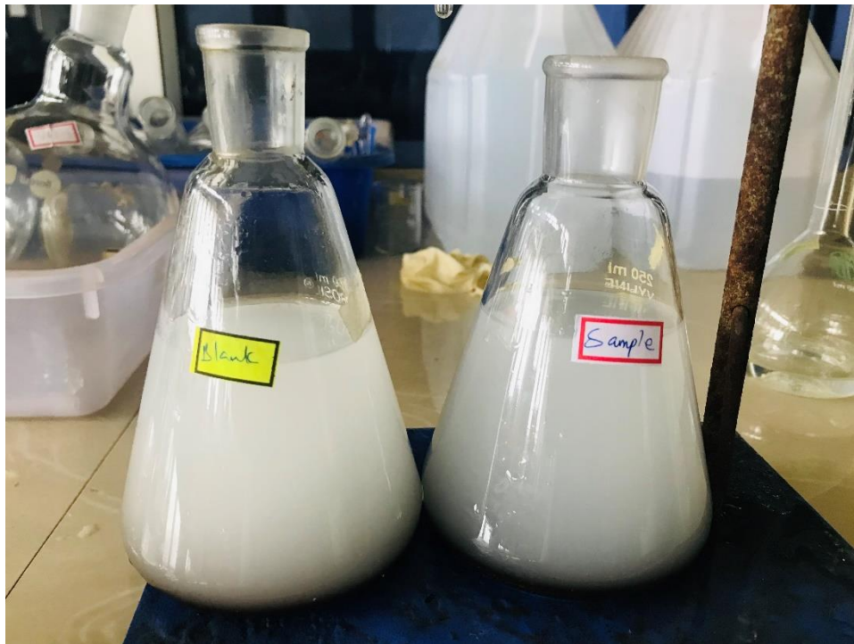
Plate 4.5. Change in colour in titration of saponification value
