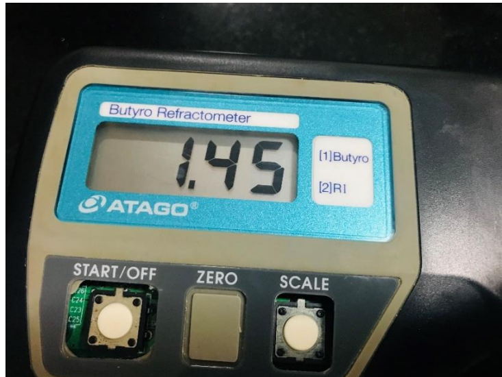
Plate 3.13. Refractometer used to measure the refractive index of Garcinia species butter
