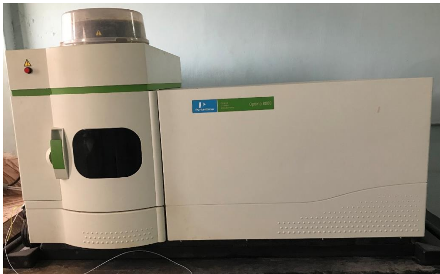
Plate 3.10. ICP- Optical emission spectrophotometer used to measure calcium and iron content
