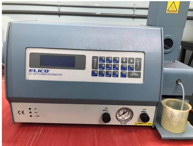
Plate 3.9. Flame photometer used to measure potassium and sodium content
