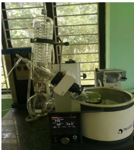
Plate 5a. Rotary evaporator
