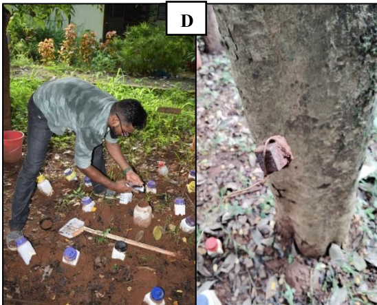
Plate 11: Images showing experimental setup for subterranean termite test A) Sample tied using galvanized wire; B) Artificial mound; C) No choice test setup; D) Recording observation; E) Termites infestation in the artificial mound; and F) Cleaning of recovered samples
