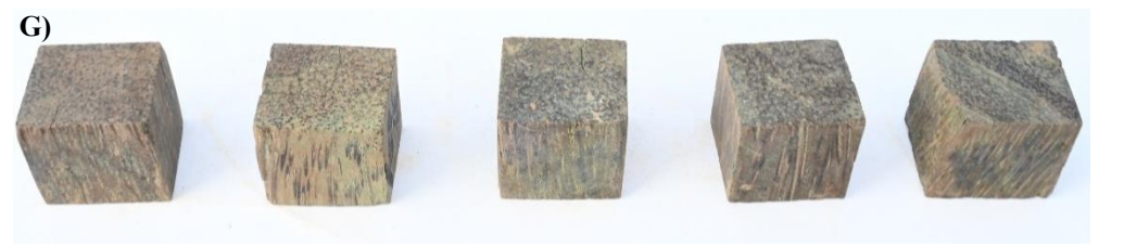
Plate 14: Effect of termite on pressure treated with nanoparticles to medium density coconut wood after incubation for subterranean termite test
