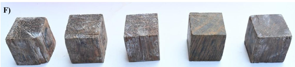
Plate 14: Effect of termite on pressure treated with nanoparticles to medium density coconut wood after incubation for subterranean termite test
