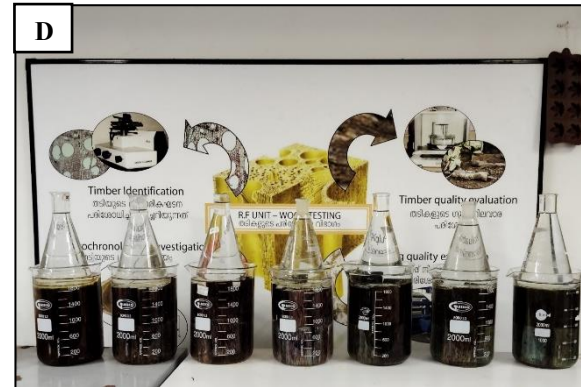
Plate 12B: Water absorption test experimental setup
