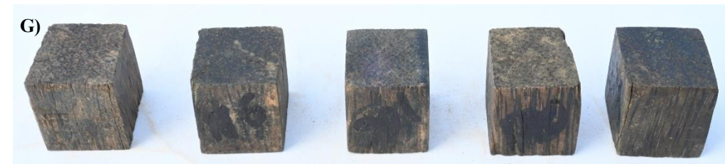
Plate 17: Effect of termite on pressure treated with nanoparticles to high density coconut wood after incubation for subterranean termite test
