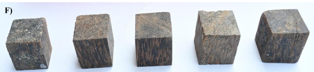
Plate 17: Effect of termite on pressure treated with nanoparticles to high density coconut wood after incubation for subterranean termite test
