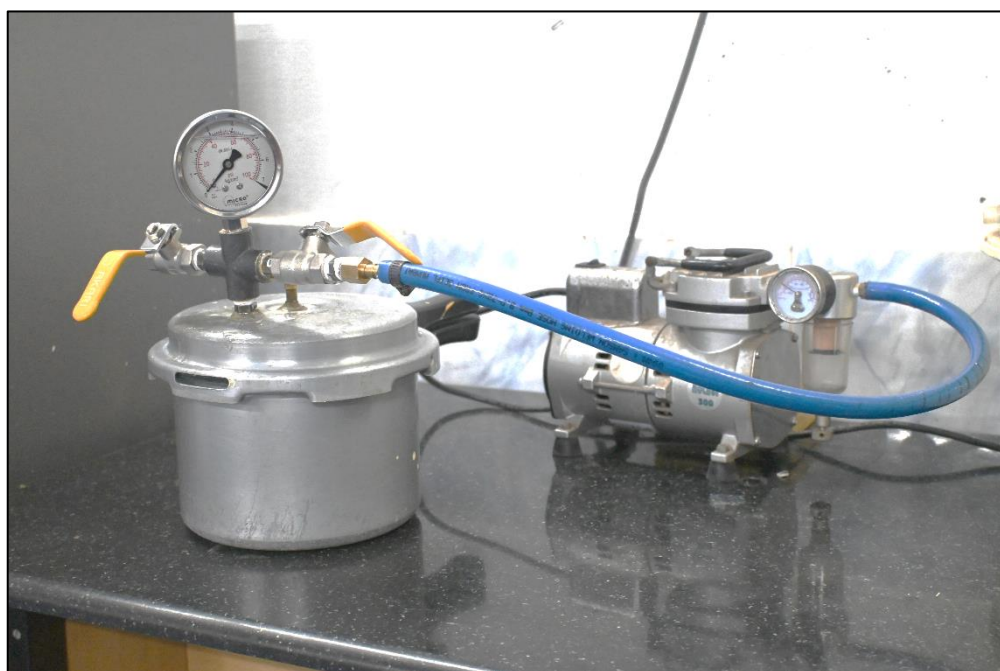
Plate 7C: Pressure treatment plant designed and used for the study
