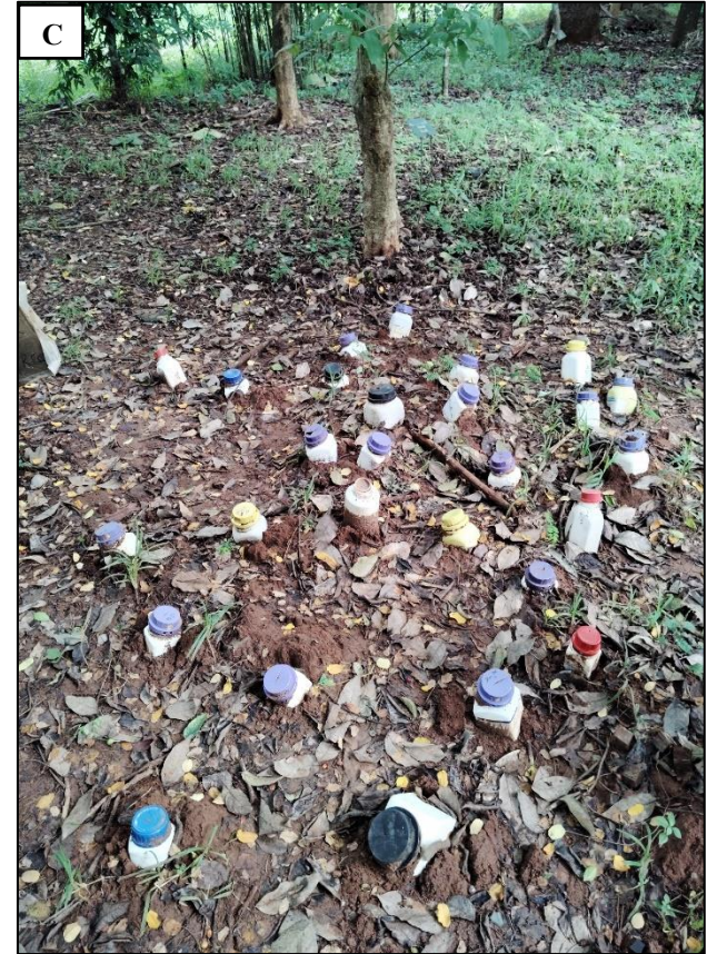
Plate 11: Images showing experimental setup for subterranean termite test A) Sample tied using galvanized wire; B) Artificial mound; C) No choice test setup; D) Recording observation; E) Termites infestation in the artificial mound; and F) Cleaning of recovered samples
