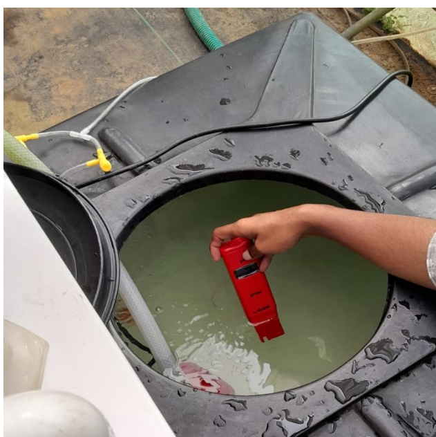
Plate 3.23 Measuring of pH of nutrient solution using HANNA portable pH meter
