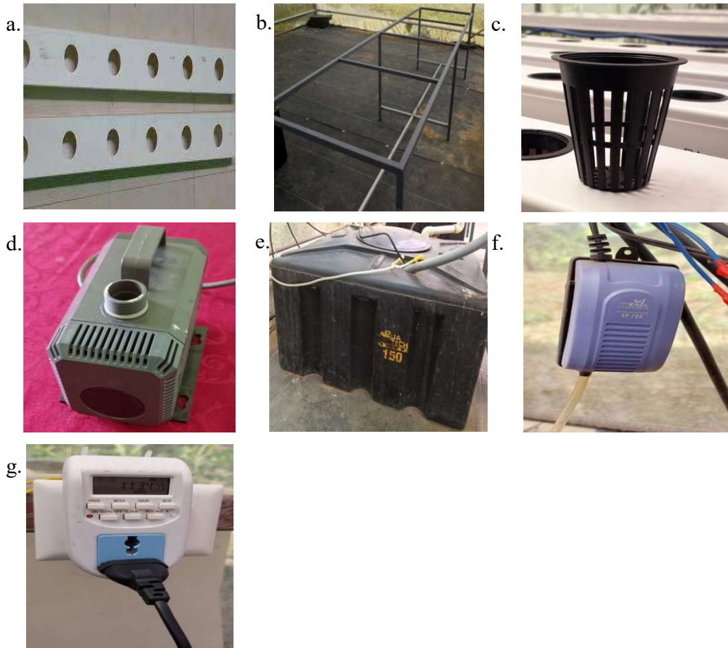
Plate 3.1 Components of NFT hydroponics system: (a) NFT channels, (b) Rack, (c) Net cup, (d) Pump, (e) Nutrient solution tank, (f) Aerator, (g) Timer
