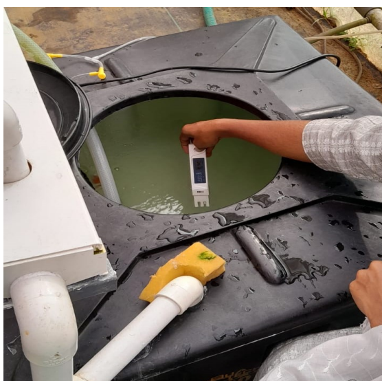
Plate 3.22 Measuring of TDS of nutrient solution using AP-1 TDS meter
