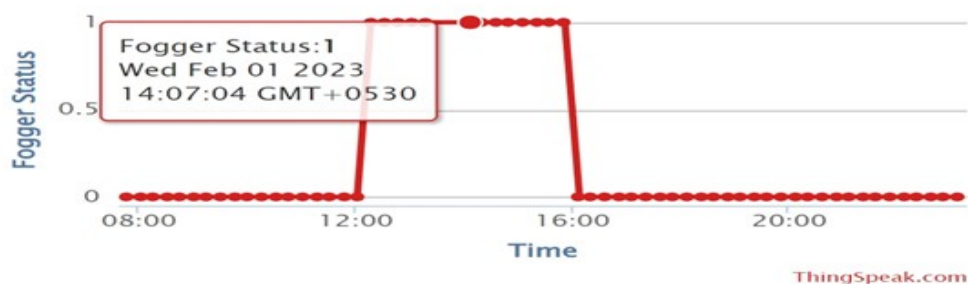
Fig. 4.38 Monitoring of real time operation status of foggers in computer from ThingSpeak IoT cloud
