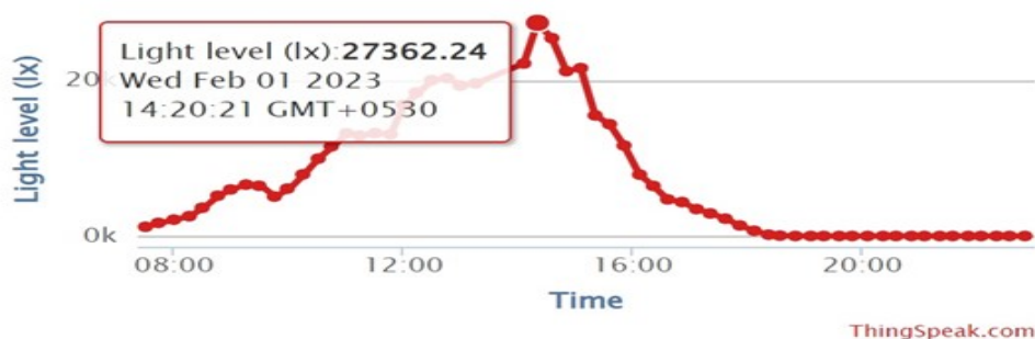
Fig. 4.35 Monitoring of real time light intensity in computer from ThingSpeak IoT cloud
