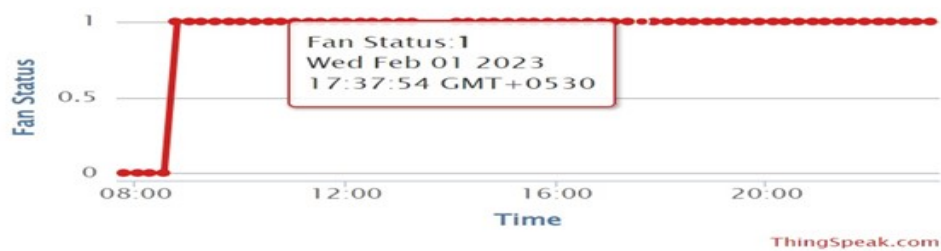
Fig. 4.37 Monitoring of real time operation status of fans in computer from ThingSpeak IoT cloud
