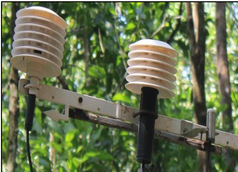
Plate 3. Sensors (Emcon Pvt. Ltd, Cochin) used for measurement of temperature, humidity and PAR
