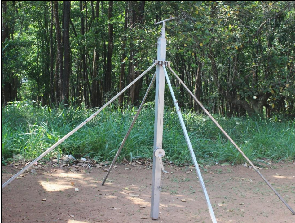
Plate 2. Micrometeorological stand fabricated to take measurement at different heights above the ground level
