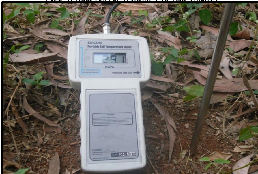
Plate 5. Soil temperature sensor (Emcon Pvt. Ltd, Cochin) used for measurement of soil temperature
