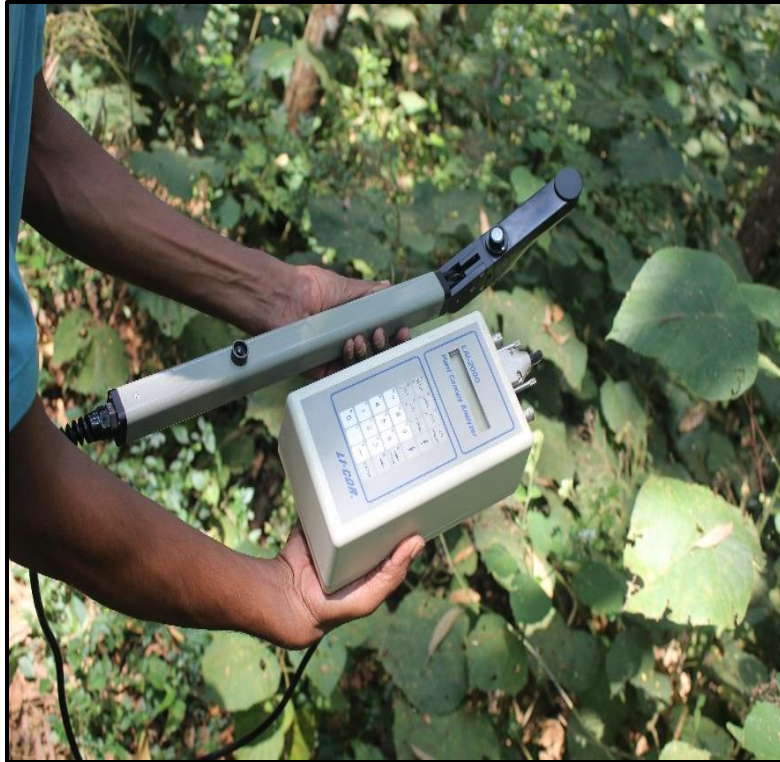
Plate 9. Canopy Analyser (LAI-2000, LI-COR Inc., Nebraska, USA) used for measurement of stand leaf area index
