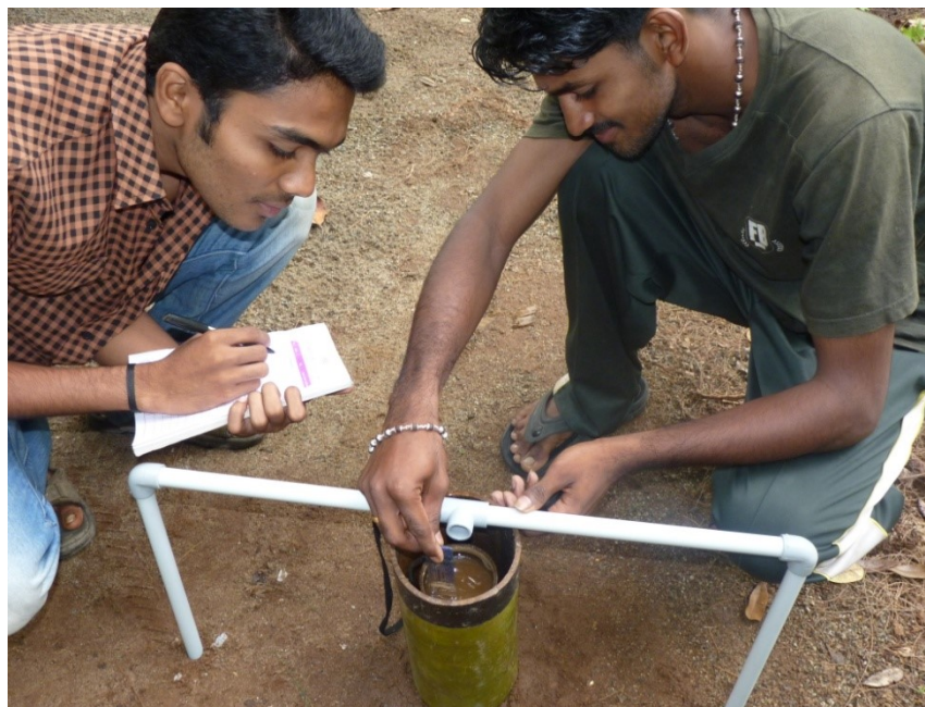
(b) Measuring infiltration rate using Double Ring infiltrometer
