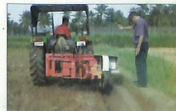
The Ridge Plastering machine in operation
