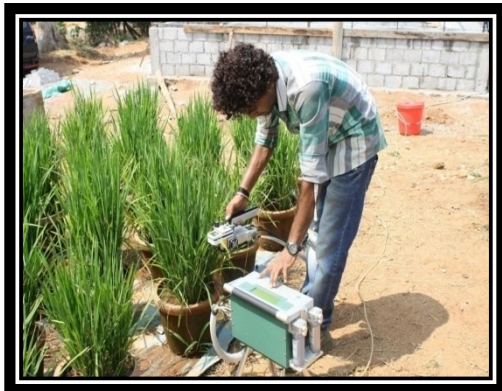
c. LI-6400 Portable Photosynthesis system
