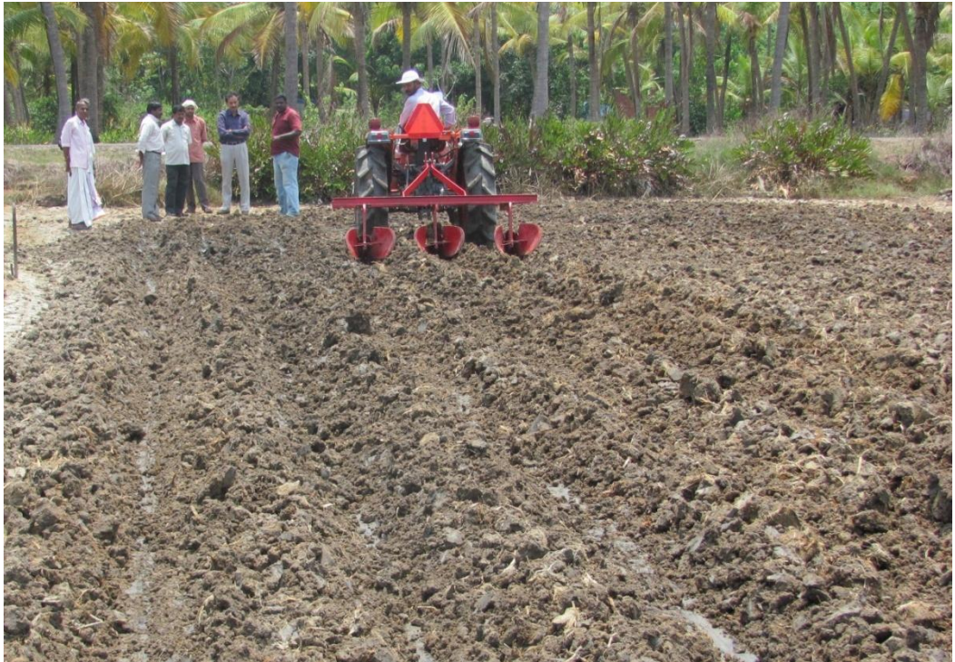
Plate. 3. 6. Field performance of tractor operated conventional ridger
