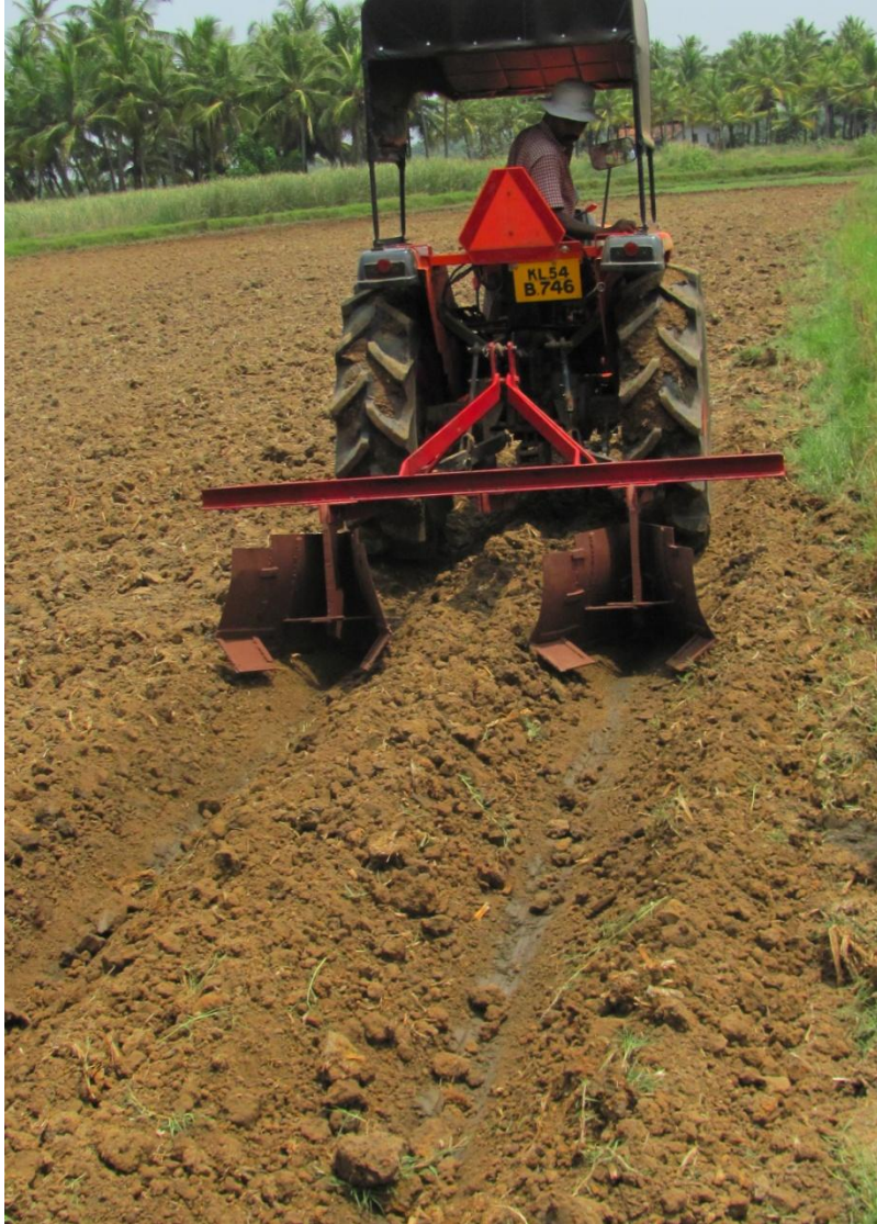
Plate. 3. 5. Field performance of tractor operated Kaipadbed former
