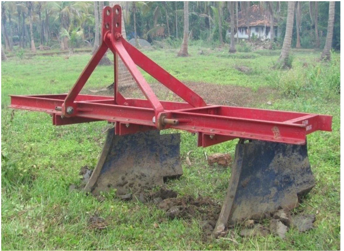
Plate. 3. 2. Tractor operated Kaipad bed former
