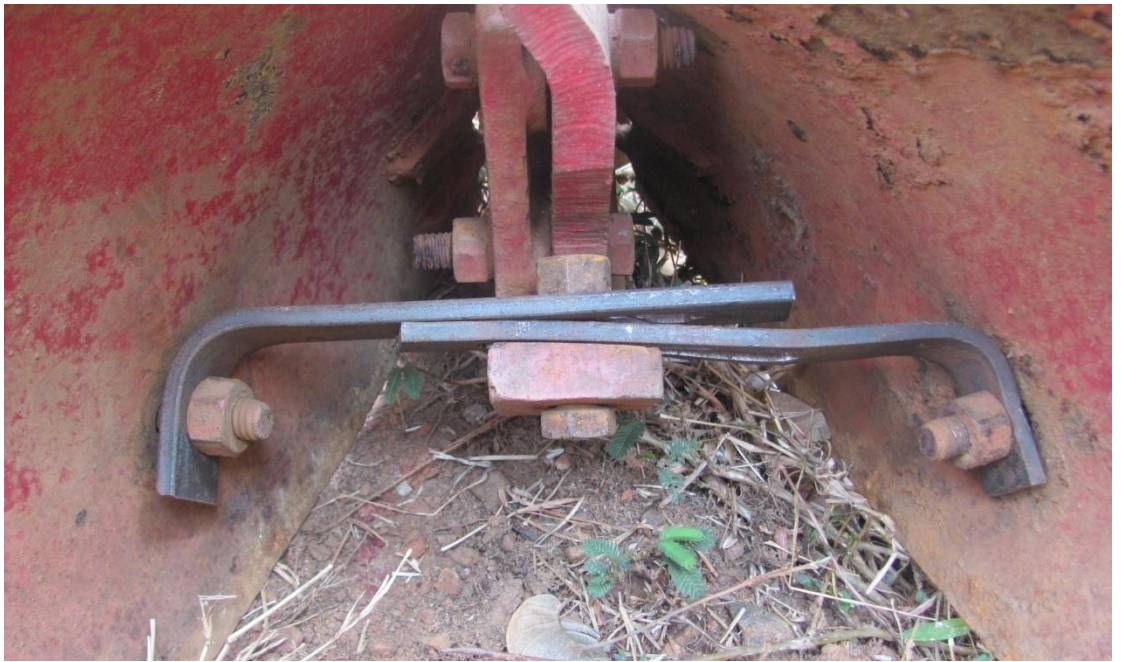
Plate. 3. 3. Angle adjustment of the plough bottom
