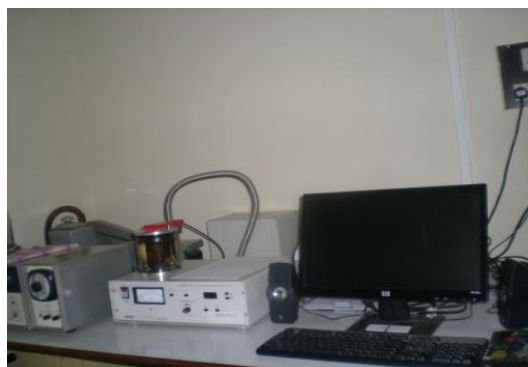
Plate 3.5 JFC – 1200 Auto fine coater (Part of SEM set up)
