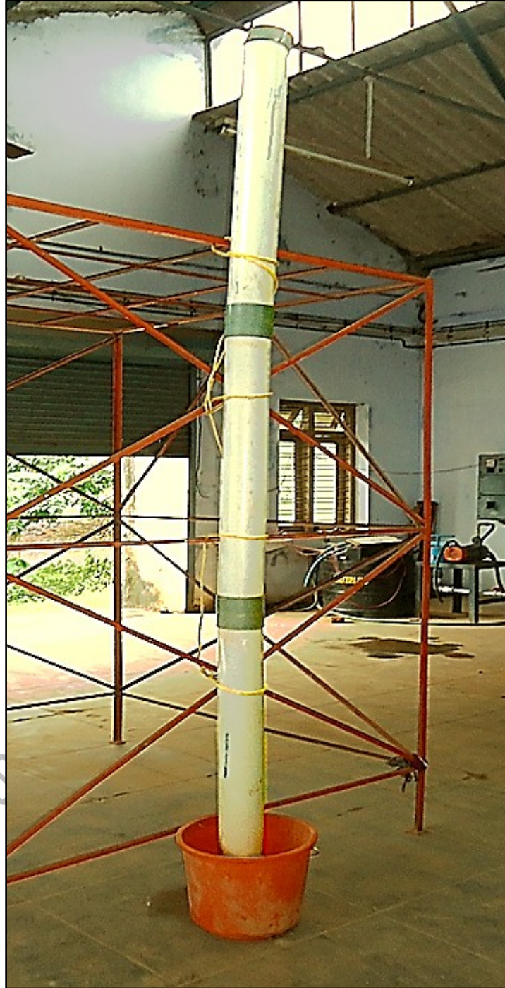
Plate 3.1 Experimental setup for determining the Wetting Curve
