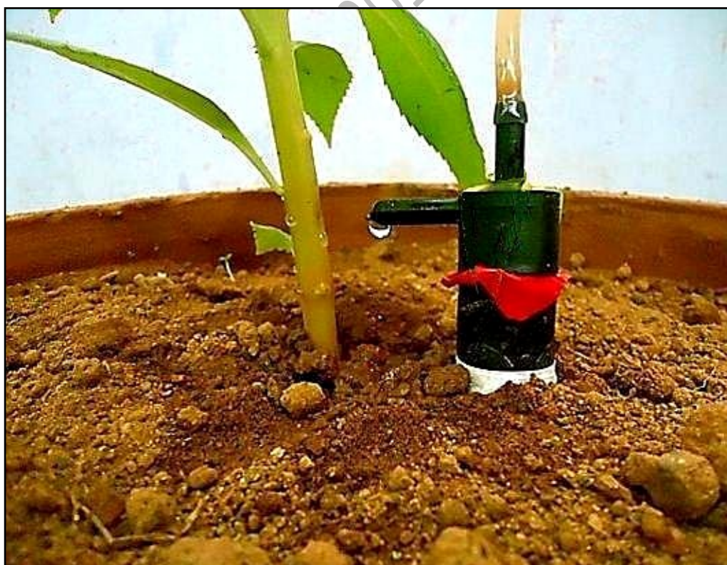
Plate 4.11 Working of the Tensio-Emitter
