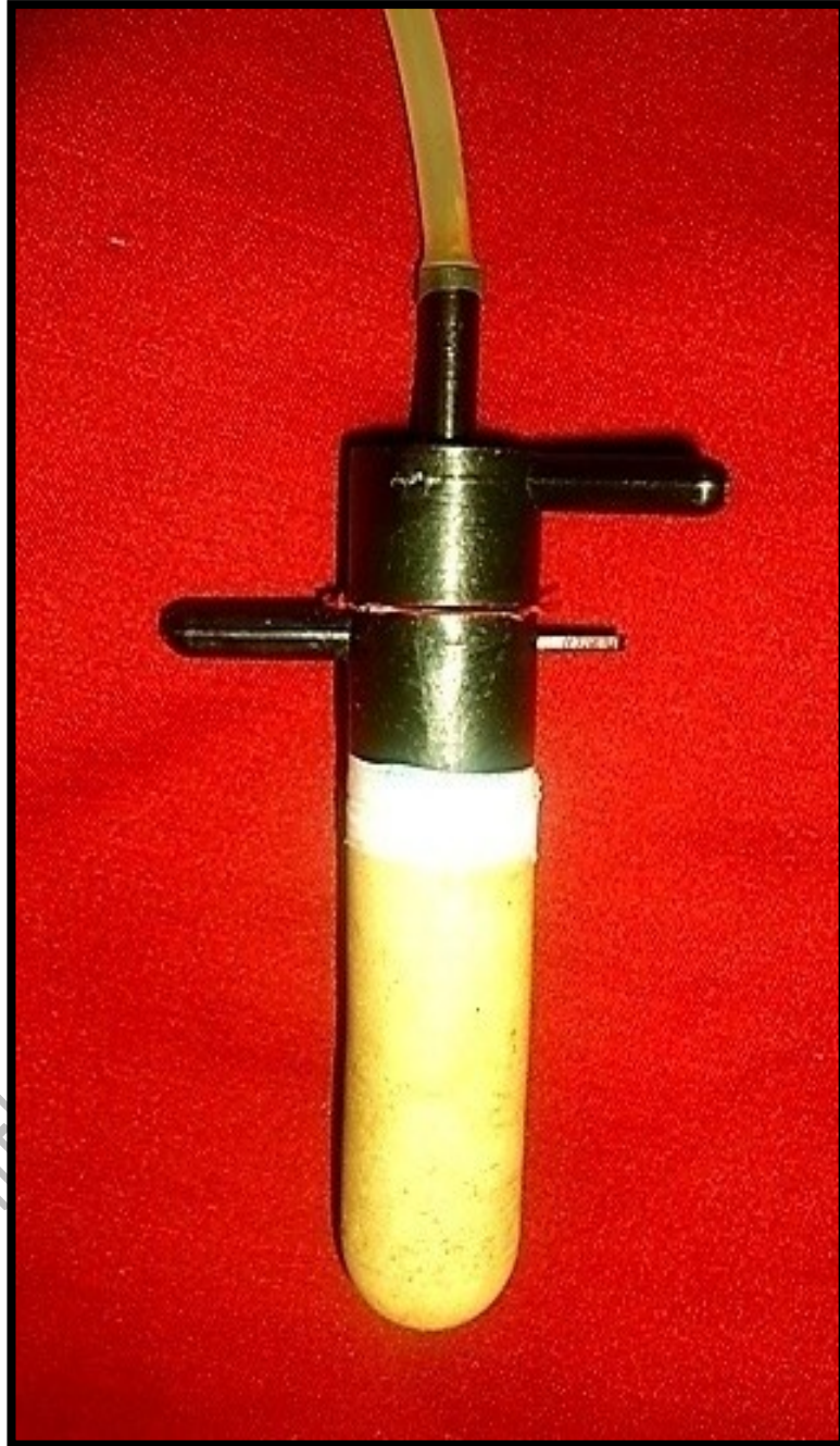
Plate 4.10 Assembled view of Tensio-Emitter
