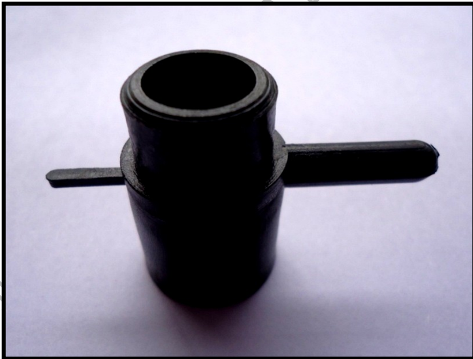
Plate 4.6 Bottom part of the emitter
