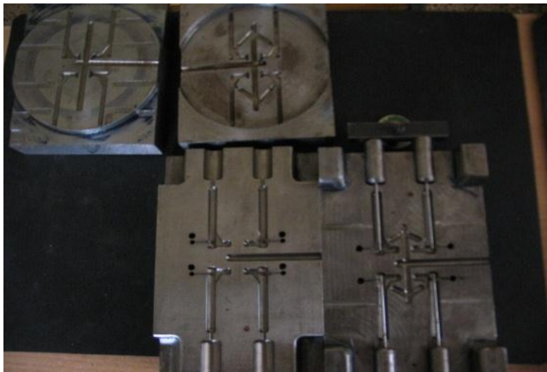
Plate 4.1 Mould developed for plastic injection moulding
