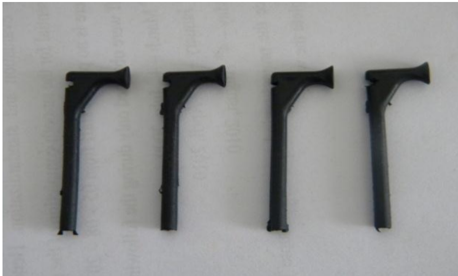
Plate 4.2 First Moulded Micro Sprinkler (FMMS)
