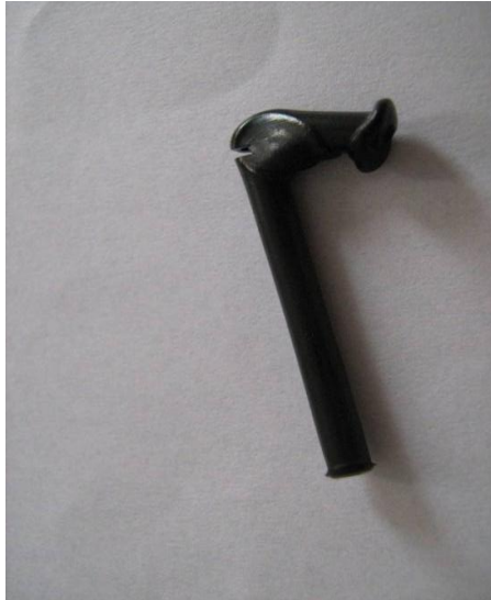
Plate 3.1 Micro sprinkler developed by the farmer
